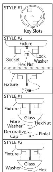
Style #1: Tuck the electrical wires into the electrical box and position the "key slots" over the support screws. Turn and lock the support screws into the "key slots". Tighten the support screws into place.
